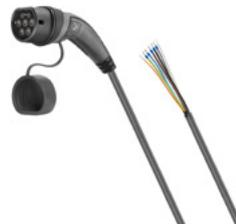
Charging cable for up to 11 kW charging power with 3-phase connection, plug type charging point: open, plug type vehicle: type 2, 10 m cable length, plug color black/grey, cable color black
