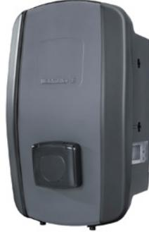
Mode 3 EV-charging box AC SMART ADVANCED, max. charging power of 22 kW at 3-phase (400 V) mains connection, maximum charging current 16 A, attached 5/7.5 m cable with type 2 plug , RFID authentication, MID compliant energy meter, integrated webserver with dynamic load management , Mobile App, Interfaces: mobile communications (4G/LTE), 2x Ethernet, WLAN, Bluetooth low energy, RS 485, 5 DI, 1 DO, powerline communication (AutoCharge)
