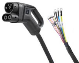
Mode 4 charging cable for up to 150 kW charging power, 150 A charging current, internal temperature monitoring, Connection charging point: open cable end, Connection to vehicle: CCS2 plug, 5m cable length, plug color black, cable colour black
