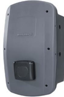
Mode 3 EV charging box AC SMART ECO, max. charging power of 22 kW at 3-phase (400 V) mains connection, maximum charging power 32 A, attached 5/7.5 m cable with type 2 plug, integrated webserver, Mobile App, Interfaces: Ethernet, WIFI, Bluetooth low energy, RS 485, 1 DI, 1 DO
