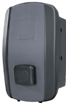
Mode 3 EV-charging box AC SMART VALUE, max. charging power of 22 kW at 3-phase (400 V) mains connection, maximum charging current 16 A, attached 5/7.5 m cable with type 2 plug, RFID-authentication, integratedt webserver with static load-charge management, Mobile App, Interfaces: 2x Ethernet, WLAN, Bluetooth low energy, RS 485, 5 DI, 1 DO
