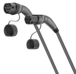
Charging cable for up to 11 kW charging capacity @ 3-phase connection, plug type charging station: type 2, plug type electrical vehicle: type 2, 7.5 m cable length, plug colour black/grey, cable colour black
